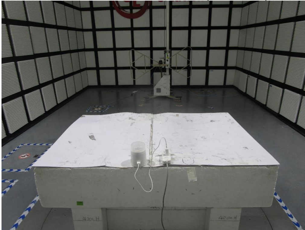
RADIATED RF MEASUREMENT SETUP (30MHz~1GHz)
