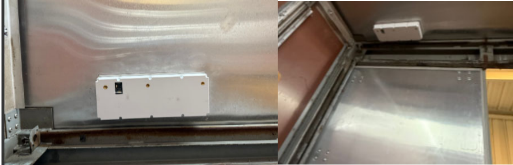
IU Flush Mounted to the Magnetic Plate
