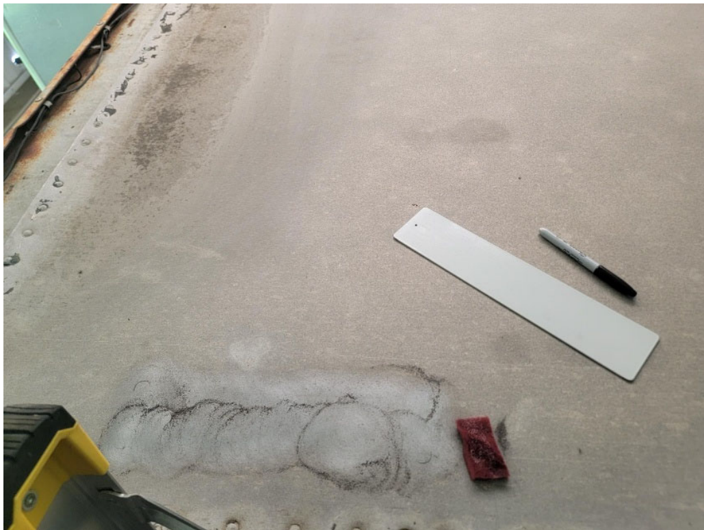
Trailer Scuffed with Oxidation Being Removed
