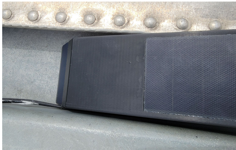
CU Mounted in C-Channel of a Trailer
