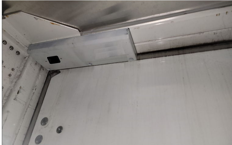
IU Mounted on Door Frame of a Trailer
