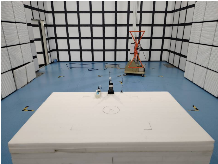
Radiation Emission - Back View (Below 1GHz)
