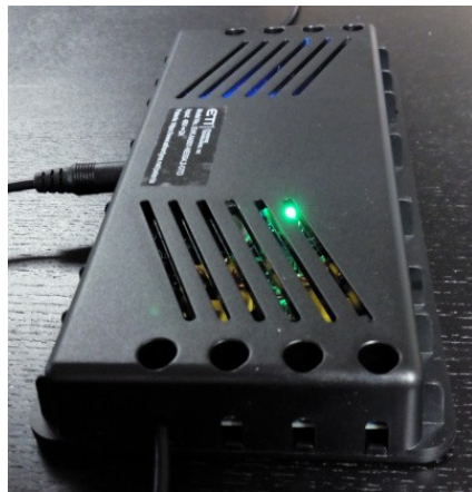
Figure 16: Green status indicator. An illuminated green LED indicates the RF Generator is operating properly and is outputting RF current.
