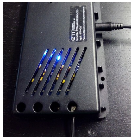
Figure 18: Yellow/Blue autotuning indicator. The color changes from yellow to blue as the tuning is changed. In shutdown mode, it glows yellow.
