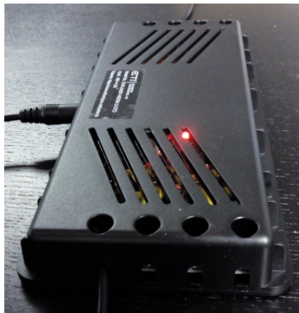
Figure 17: Red status indicator. An illuminated red LED indicates a problem has been detected and the RF Generator has automatically shut down.
