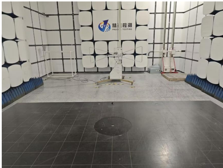
Radiated Emissions From 30M-1GHz
