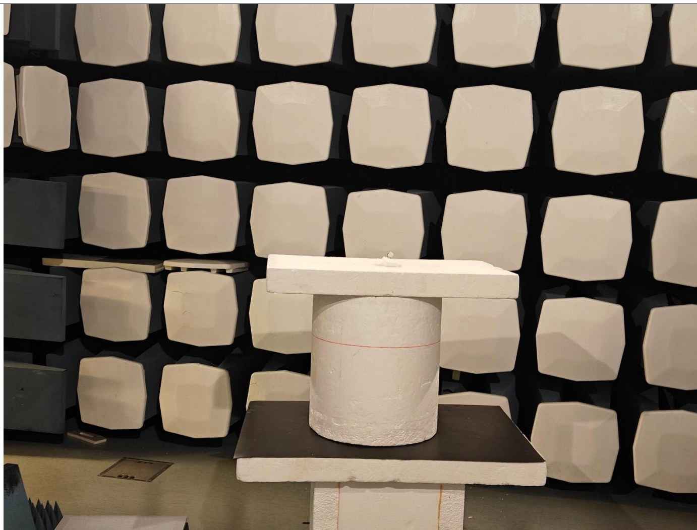
Picture 43, Radiated Spurious Emission, EUT setup, TX, 1 – 26 GHz
