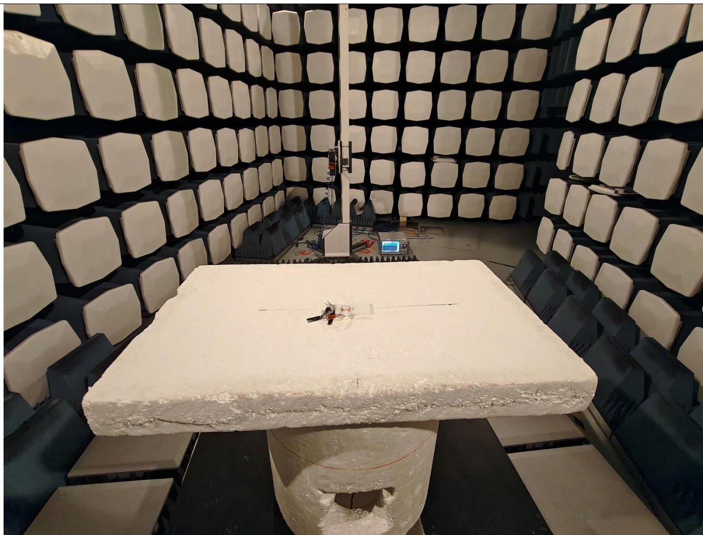
Picture 88, Radiated Spurious Emission, common setup, TX, 18 – 26 GHz, back
