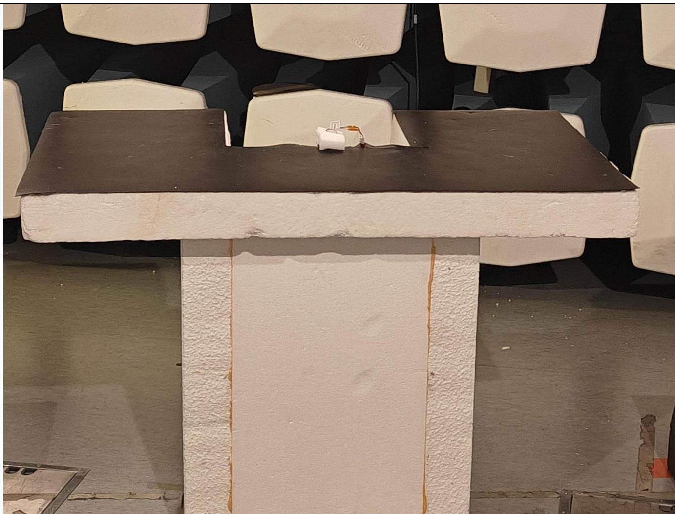
Picture 54, Radiated Spurious Emission, EUT setup, RX, 30 MHz – 18 GHz
