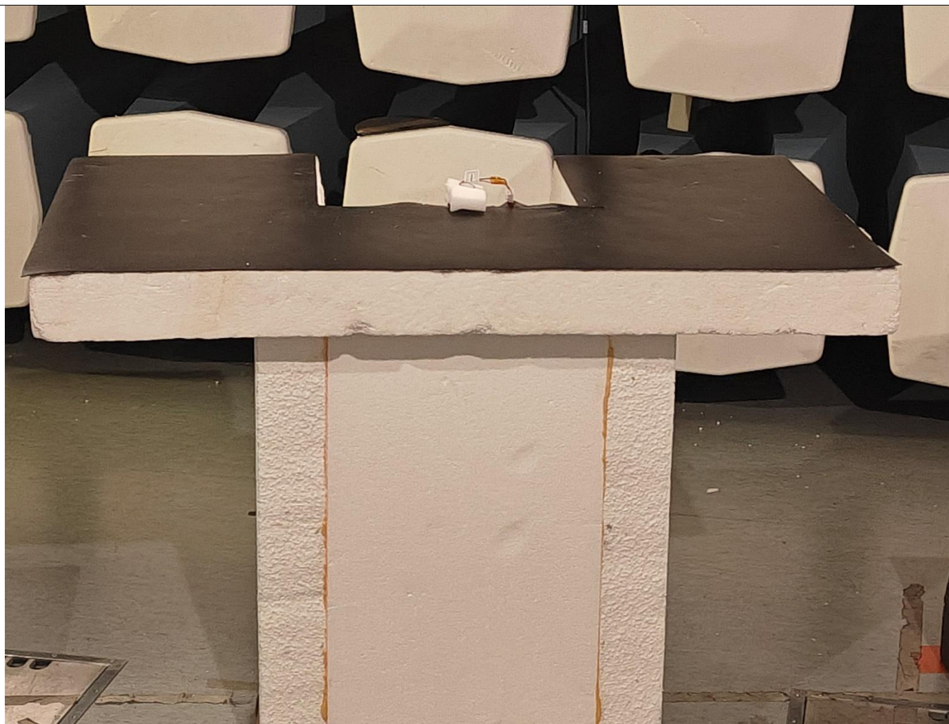
Picture 32, Radiated Spurious Emission, EUT setup, TX, 30 – 1000 MHz
