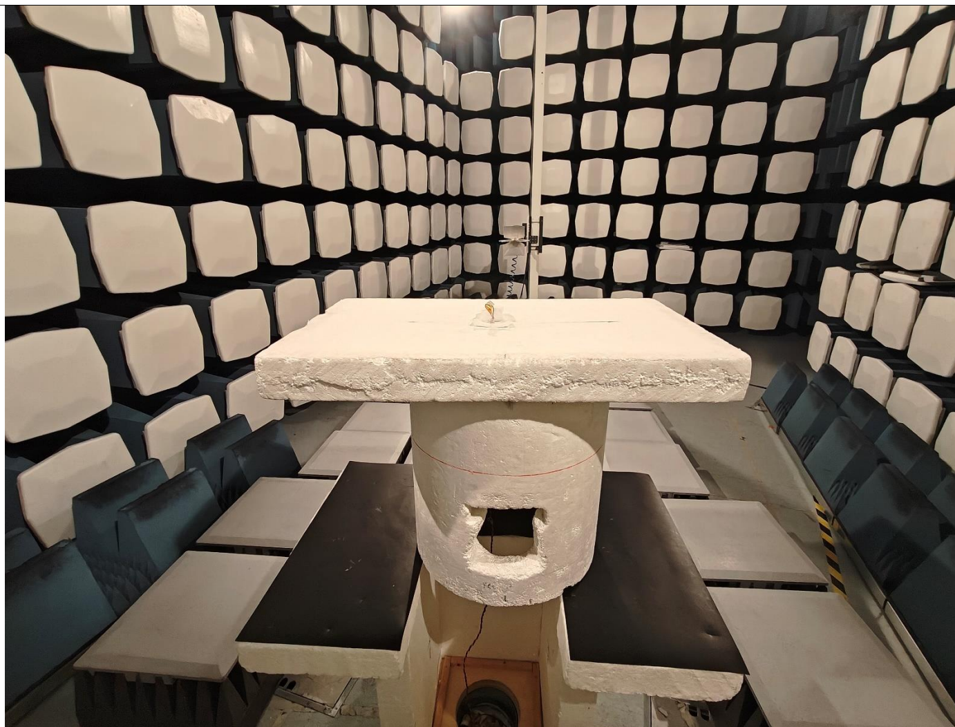
Picture 77, Radiated Spurious Emission, common setup, TX, 1 – 18 GHz, back
