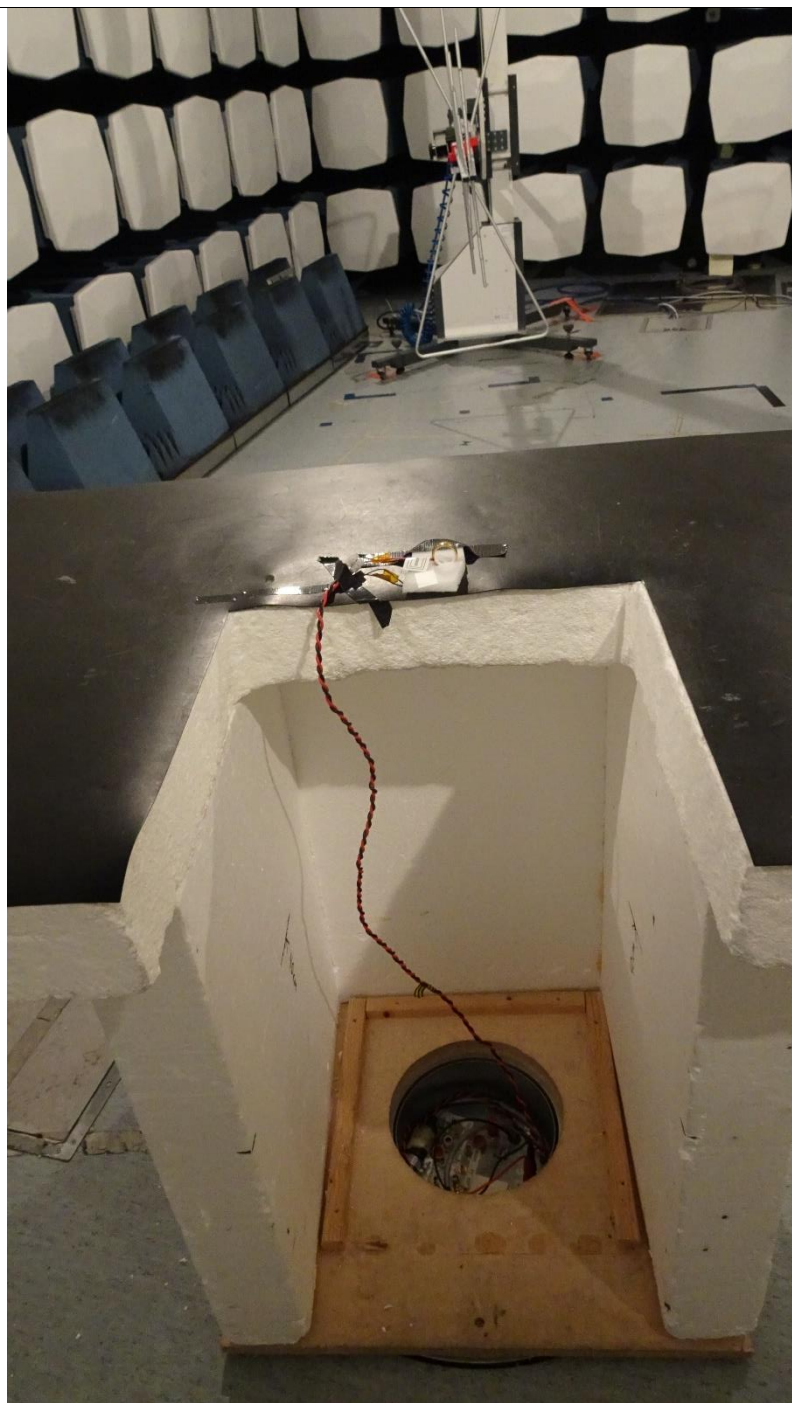
Picture 19, Radiated Spurious Emission, common setup, RX, 30 – 1000 MHz, back
