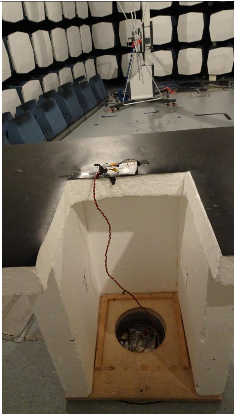
Picture 66, Radiated Spurious Emission, common setup, TX, 30 – 1000 MHz, back
