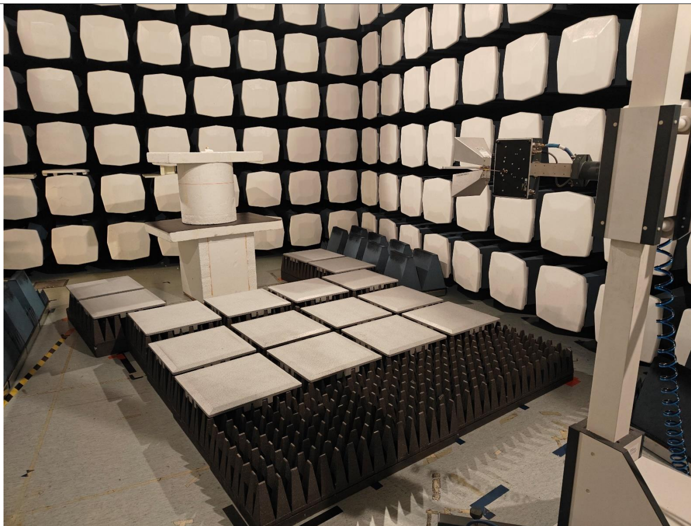
Picture 9, Radiated Spurious Emission, common setup, TX, 1 – 18 GHz, front
