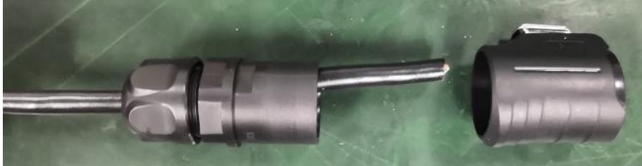
Figure 3-15 Step 1 of connecting the network cable
