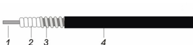
Figure 3-20 Schematic of Feeder Cable (1/4 Ultra-Flexible RF Cable)
