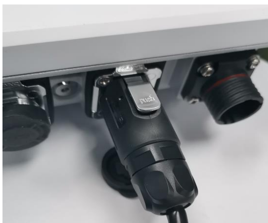
Figure 3-19 Step 5 of connecting the network cable
