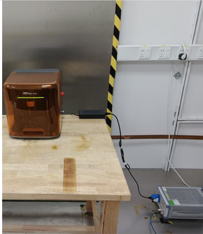
AC Power Line Conducted Emission
