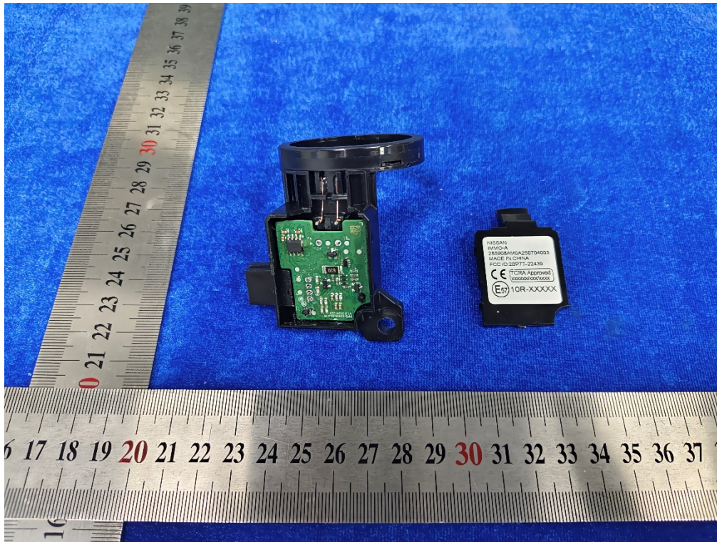
Photo 1: Internal View for PCB
