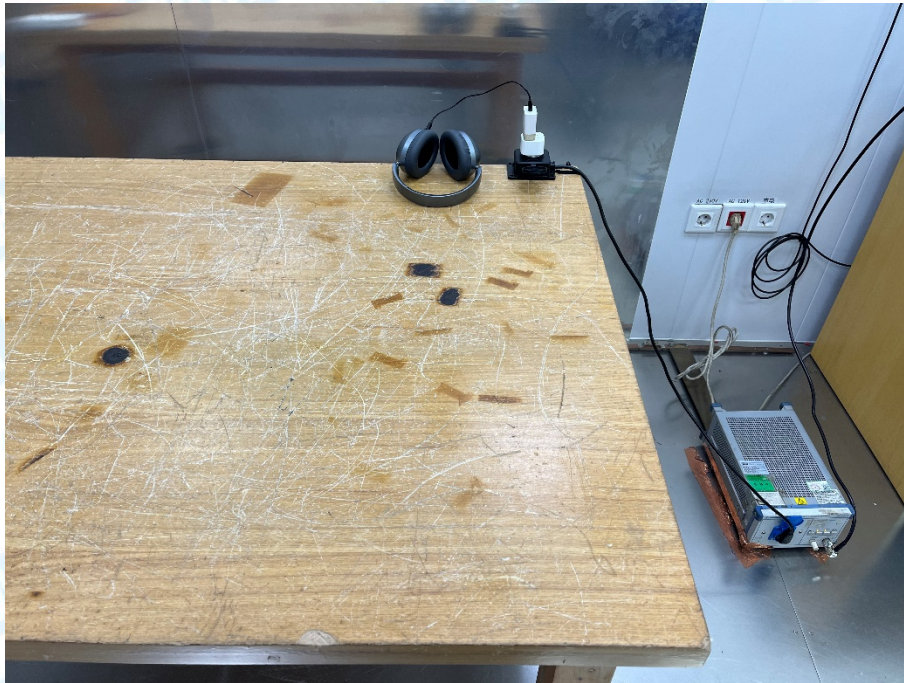
Photo of Setup for Conducted Measurement
