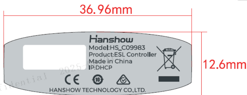
Figure 2-1 Nameplate of HS_C09983
