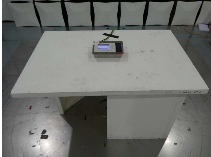
Test setup semi anechoic chamber (normal position)
