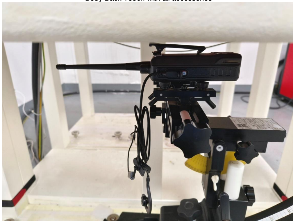
The thickness of EUT is 3.5 cm
