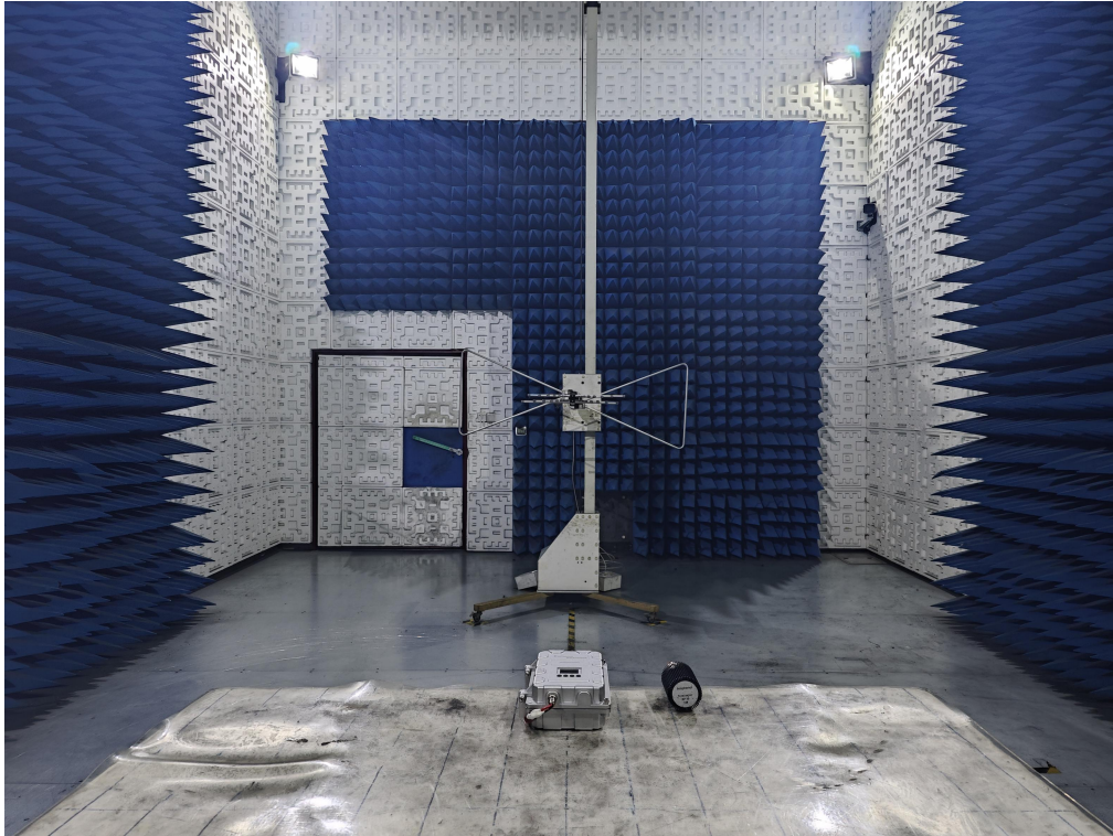
Radiated Emission Test Setup Above 1GHz (DC Power)
