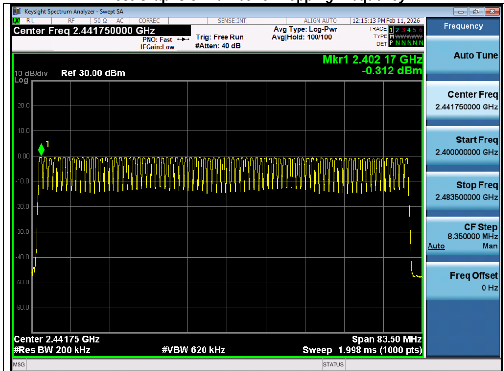
Test_Graph_BR_HOP_ANT1_NA_1Mbps_Number of Hopping
