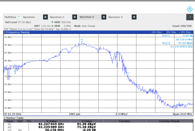
Figure 7.5-2: OBW measurement view Mid Ch
