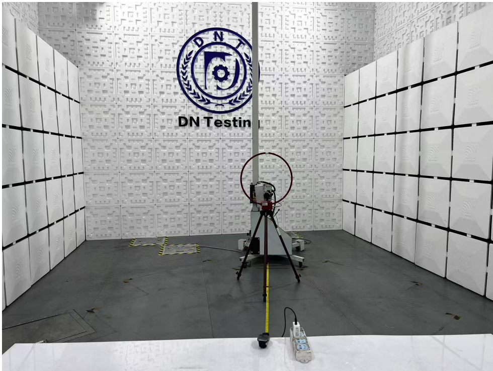
Radiated Emission Test View|(9K-30MHz)
