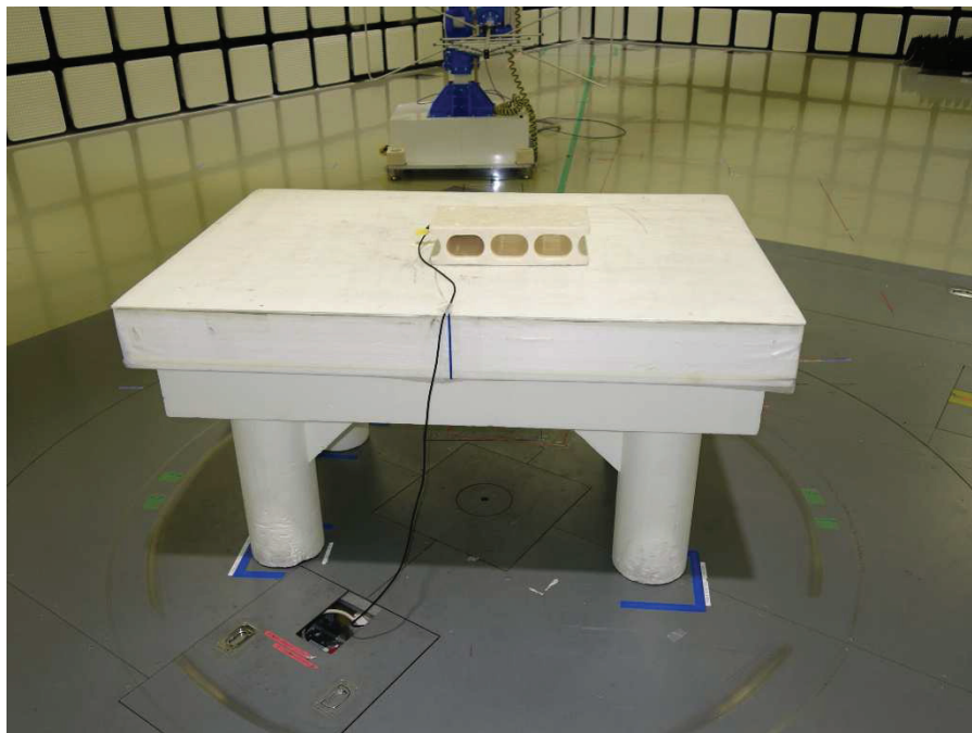
Photograph 4: Set-up for Radiated Spurious Emission below 1GHz, Rear View 1
