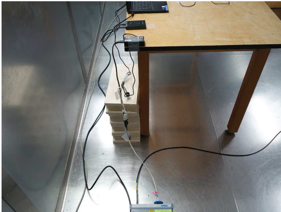
Photograph 10: Set-up for AC Power Line Conducted Emission, Rear View
