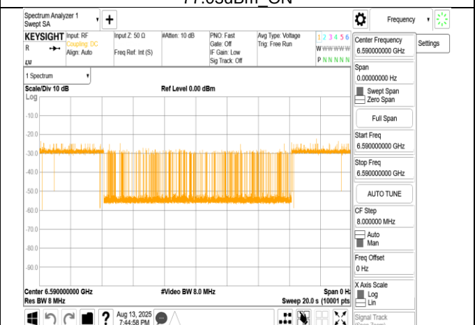
802.11ax_160MHz_CF 6665MHz_Interference_6590MHz_- 75.01dBm_Minimal
