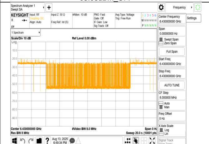
802.11ax_160MHz_CF 6505MHz_Interference_6430MHz_- 74.08dBm_ON
