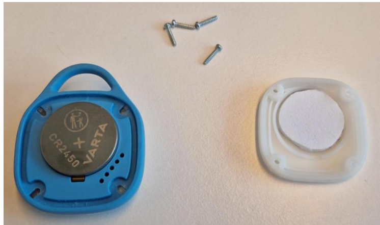
Figure 4. Opened tag with battery in place.
