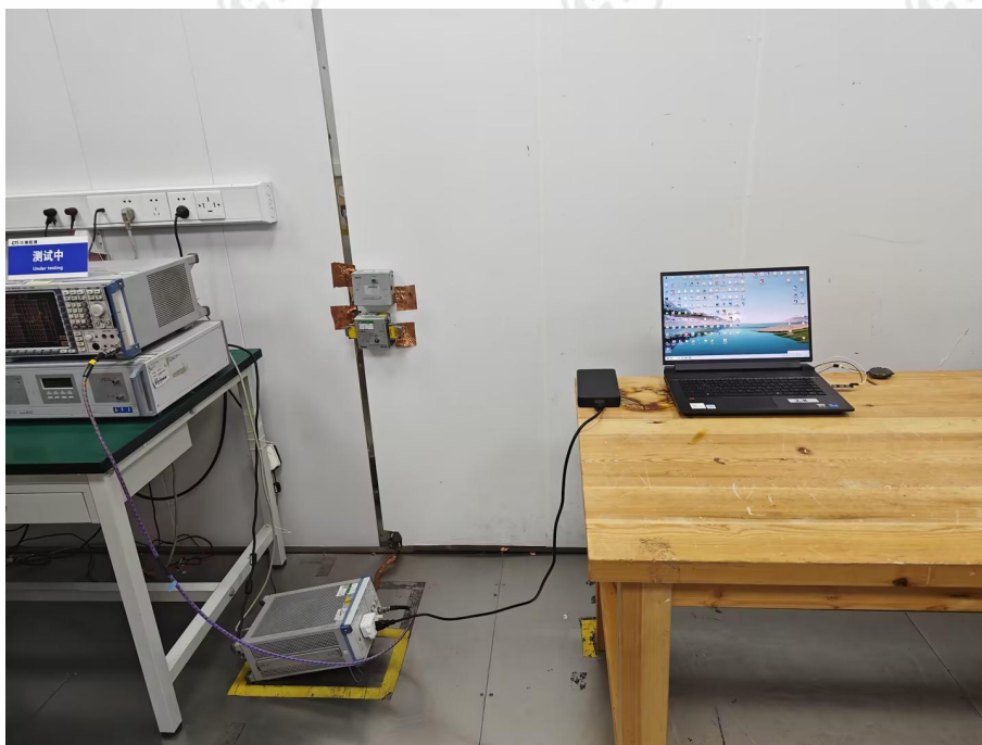
Conducted Emissions Test Setup
