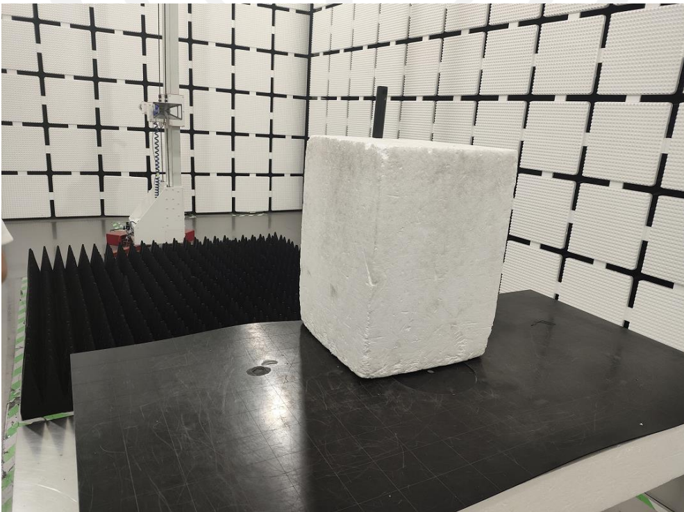
Spurious Radiation Emissions Test (>1G)
