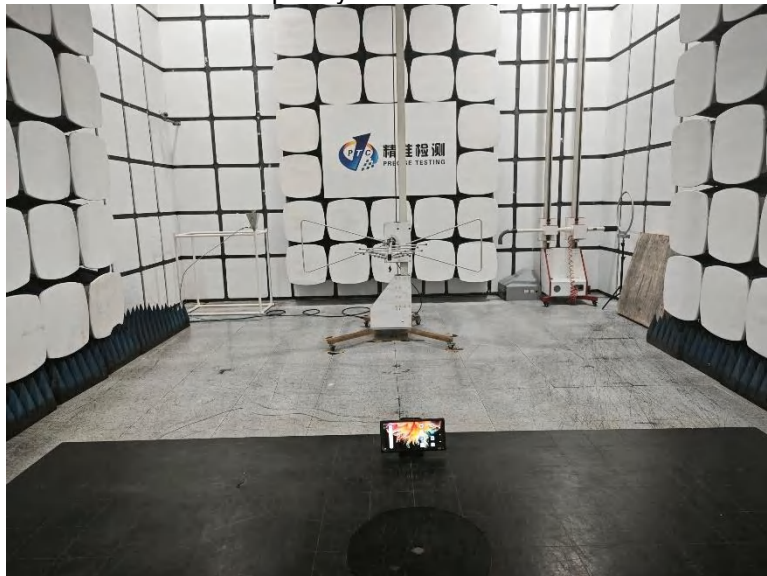
Radiated Spurious Emissions Test Frequency From 30MHz to 1GHz
