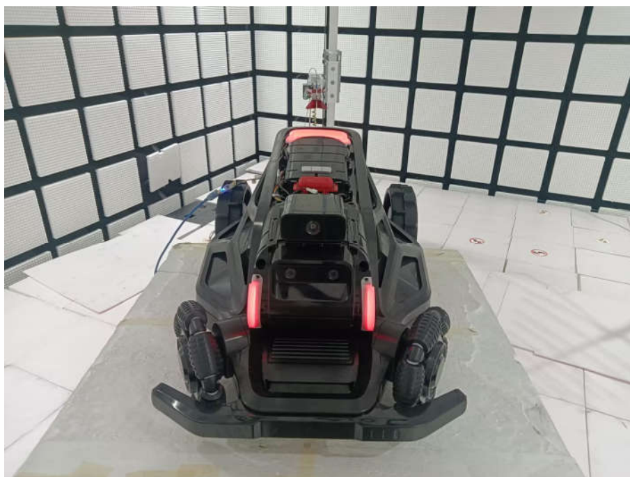
Radiated spurious emission Test Setup-2(Above 1GHz)
