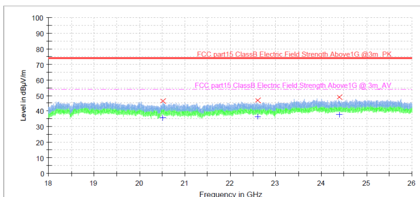
Figure 36: Spectral Diagrams, Radiated Emission, 18GHz-26GHz, Vertical, BLE 1M 2440MHz
