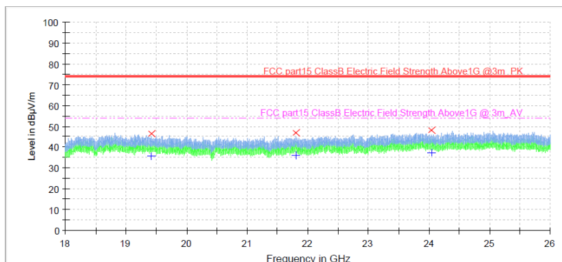
Figure 41: Spectral Diagrams, Radiated Emission, 18GHz-26GHz, Horizontal, BLE 1M 2480MHz
