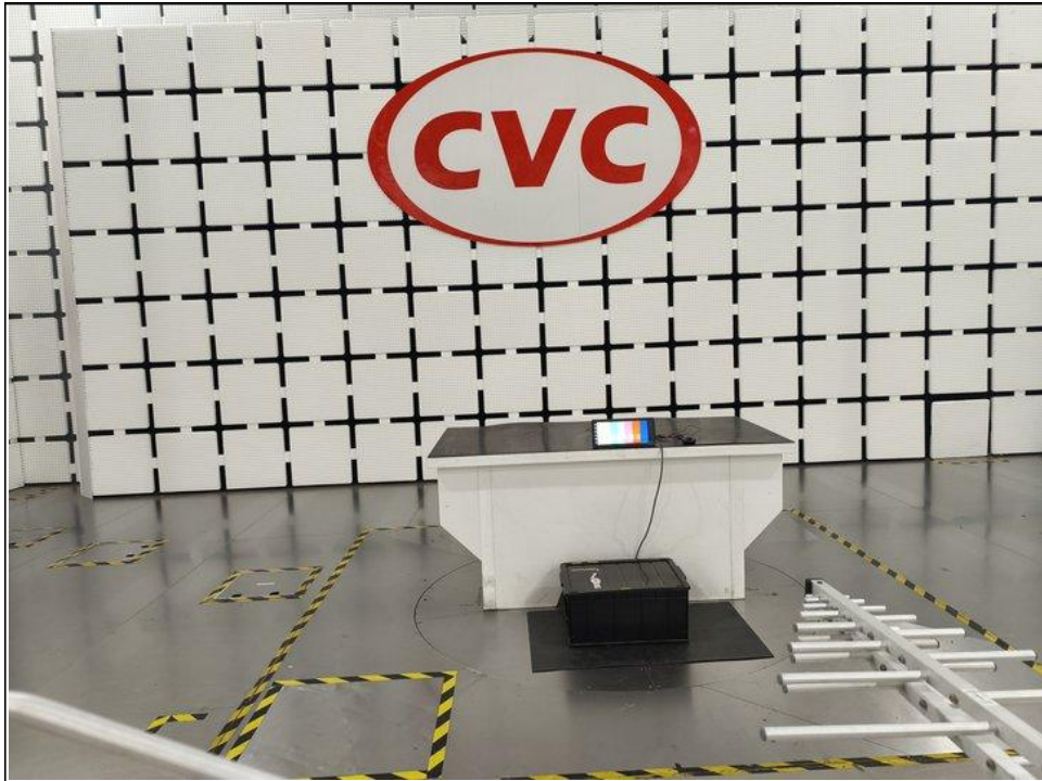
RADIATED EMISSION TEST BELOW 1GHz
