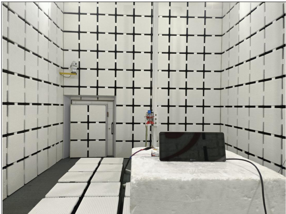
RADIATED EMISSION TEST (1GHz ~ 18GHz)
