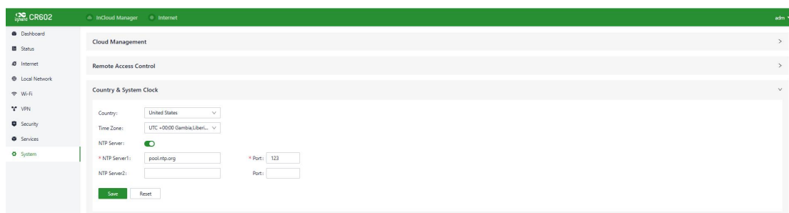
Fig. 5-9-3 Set the System Clock and NTP Server
