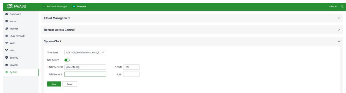
Fig. 5-9-3 Set the System Clock and NTP Server
