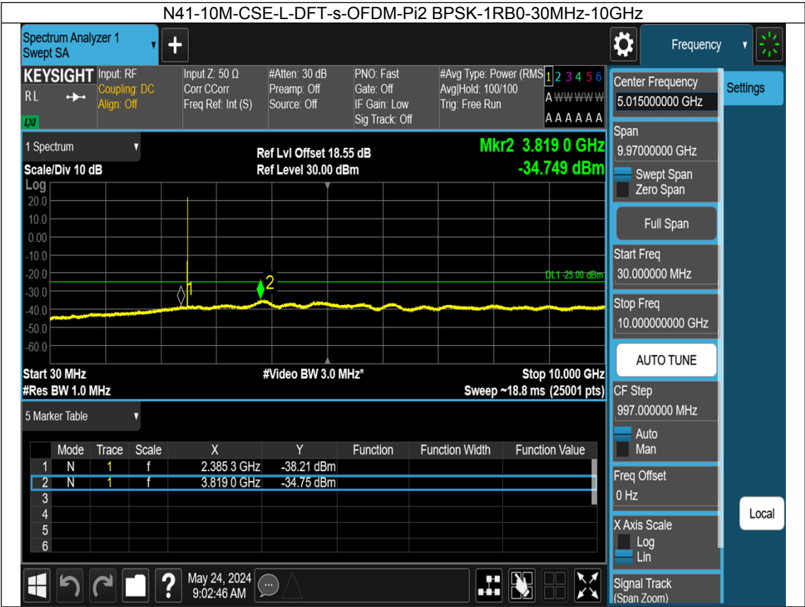
Conducted spurious emissions test graph
