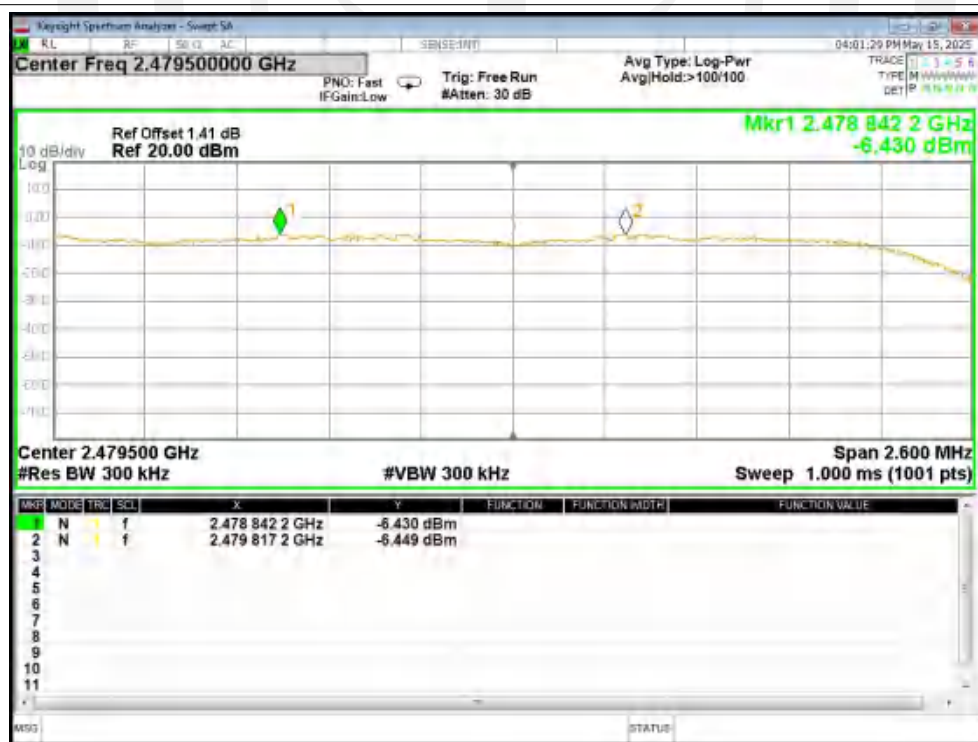
CFS NVNT 2-DH5 2480MHz Ant1
