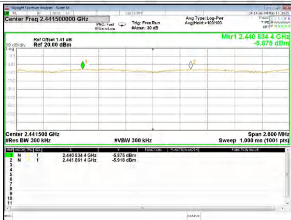
CFS NVNT 3-DH5 2441MHz Ant1
