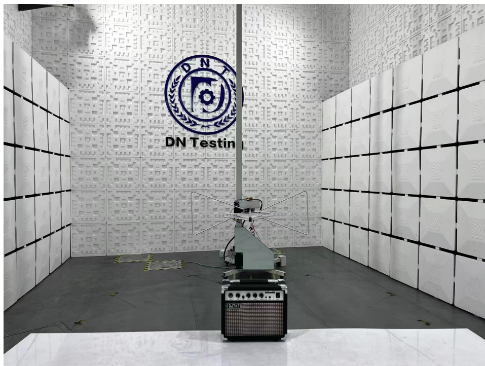
Radiated Emission Test View|(Below 1G)
