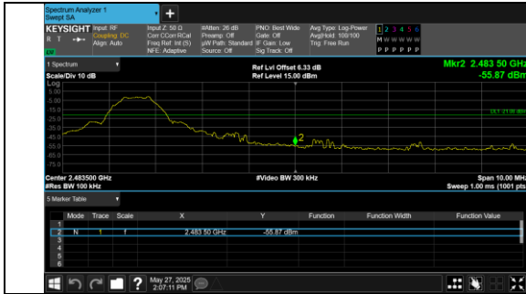
Out Of Band Emission BLE 1M_Channel 39
