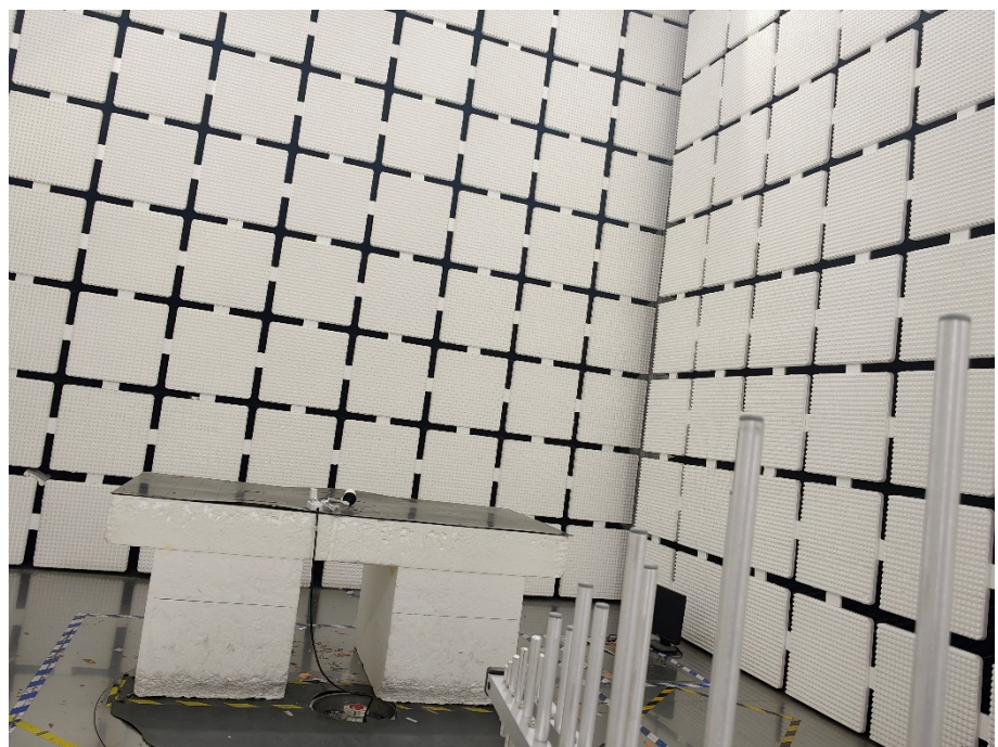
Radiation Emission Test Setup (30MHz to 1GHz)
