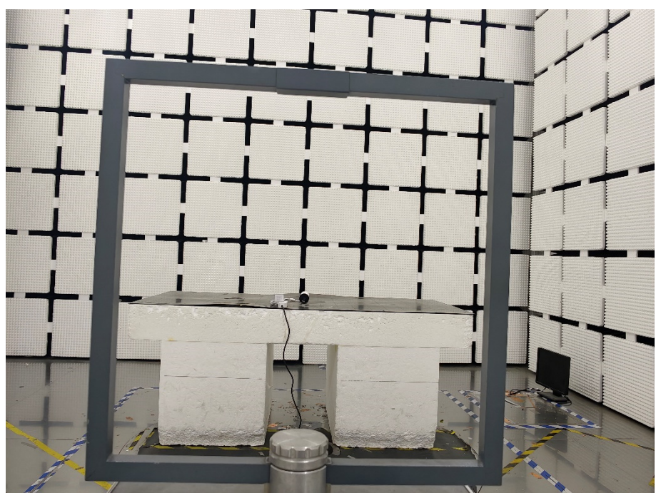
Radiation Emission Test Setup (Below 30MHz)
