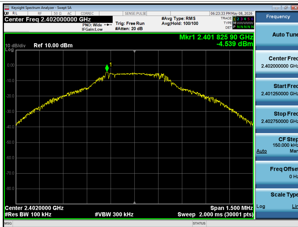
Tx. Spurious NVNT 1-DH5 2402MHz Ant1 Ref
