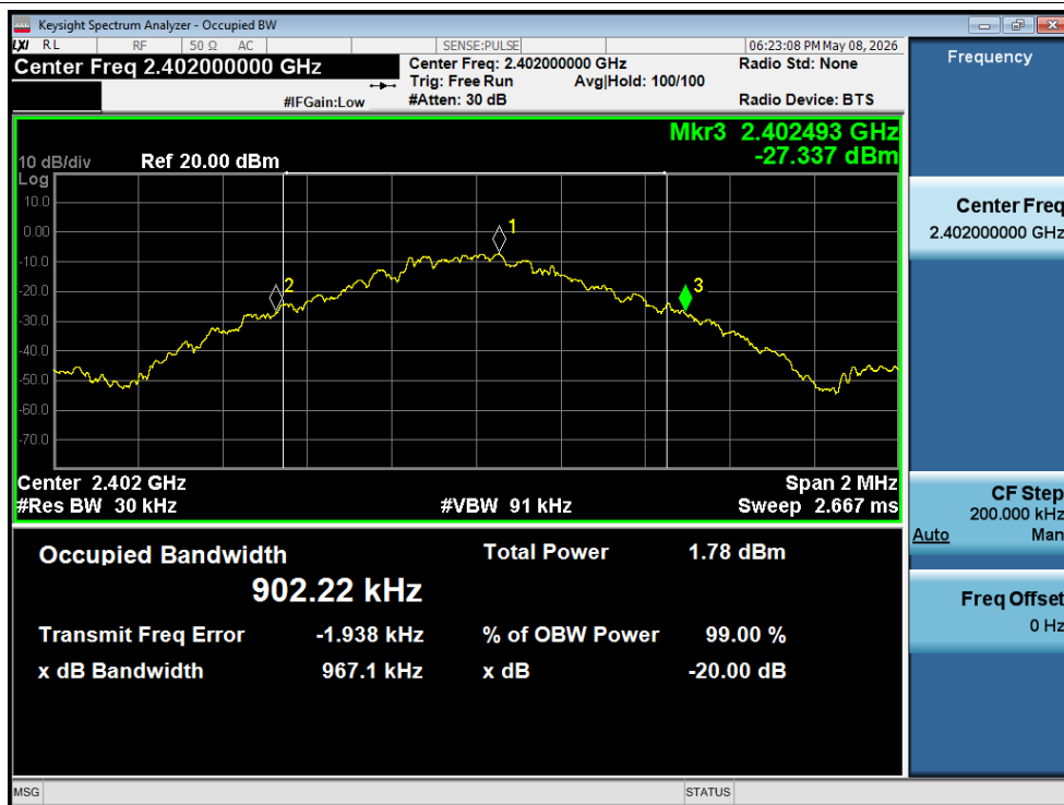
-20dB Bandwidth NVNT 1-DH5 2402MHz Ant1
