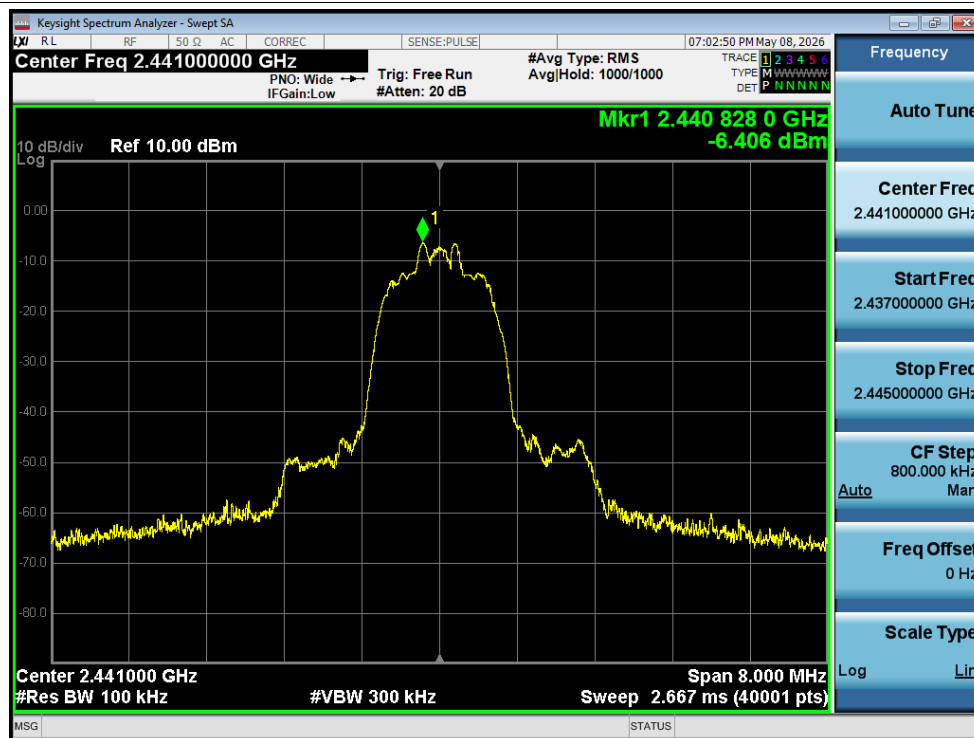
Tx. Spurious NVNT 3-DH5 2441MHz Ant1 Ref
