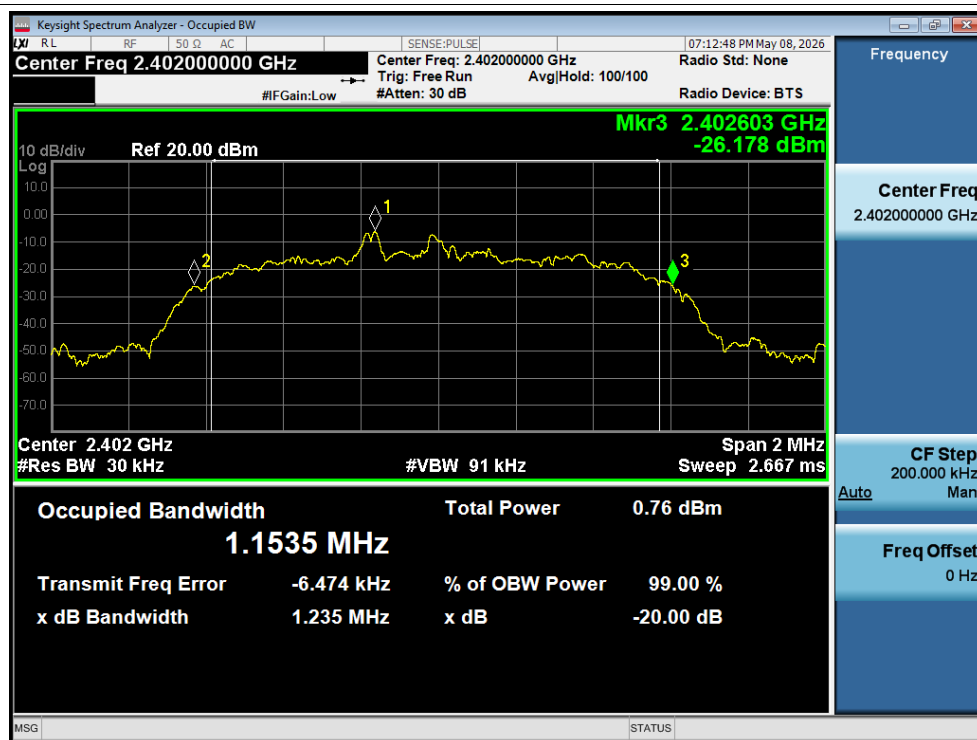
-20dB Bandwidth NVNT 3-DH5 2402MHz Ant1
