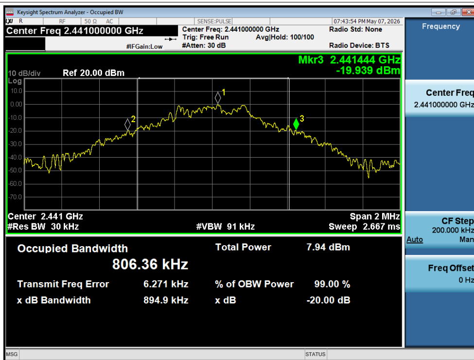
-20dB Bandwidth NVNT 1-DH5 2441MHz Ant1
