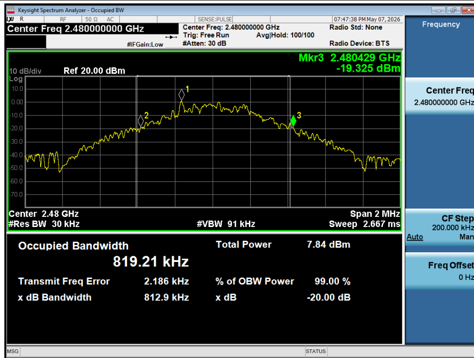
-20dB Bandwidth NVNT 1-DH5 2480MHz Ant1
