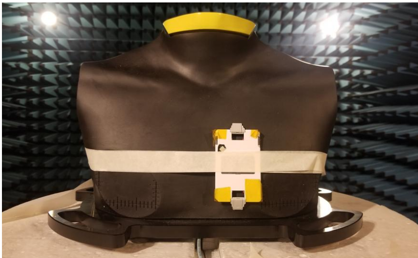
Figure 4 - DUT positioned on test phantom
