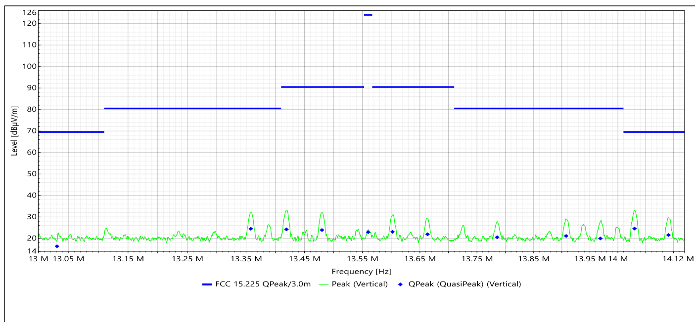
Figure 2.4.6-2 – Radiated Field Strength of Emissions within the 13.110-14.010 MHz Band
