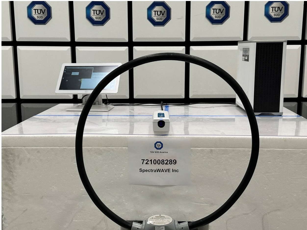
EIRP measurement at 1 meter
