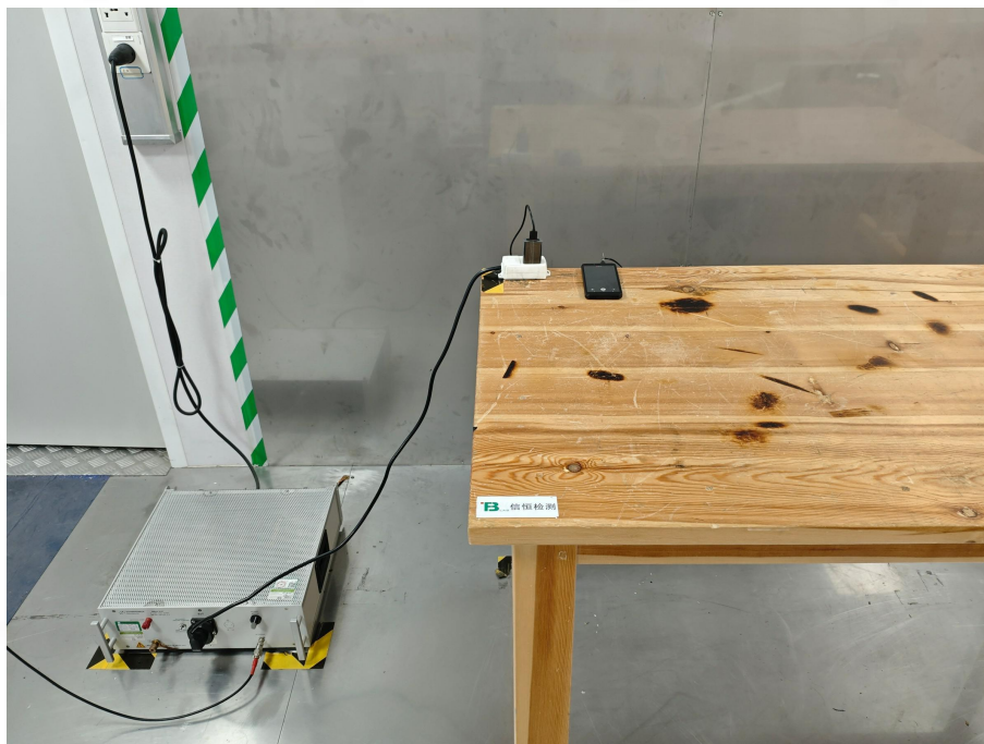
Conducted Emission at AC power line
