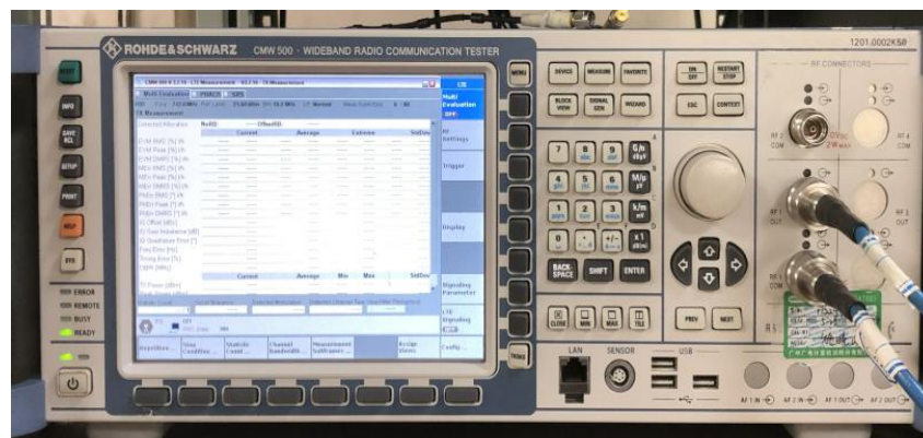
CMW 500 (2G/3G/4G Test Equipment)
