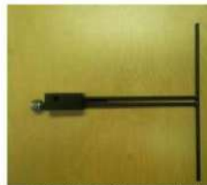
Figure 1 – MVG COMOSAR Validation Dipole
