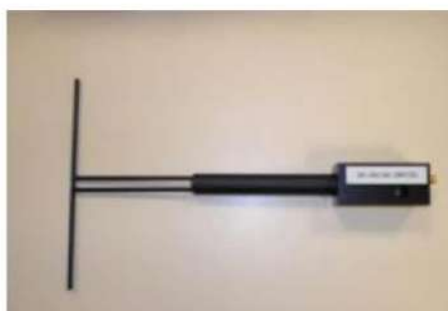
Figure 1 – Satimo COMOSAR Validation Dipole
