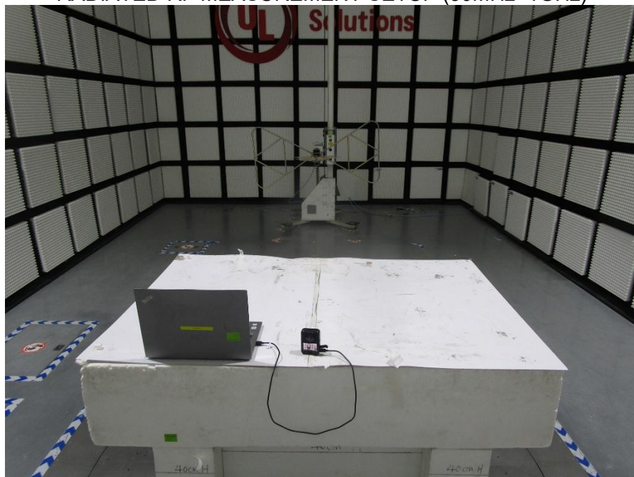
RADIATED RF MEASUREMENT SETUP (30MHz~1GHz)
