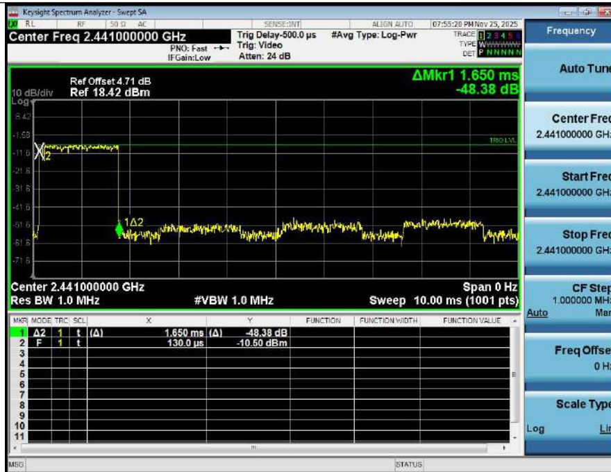
Dwell Time (Hopping) NVNT_ANT1_2-DH3_2441_00_Accumulated
