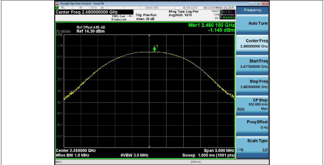
Peak Output Power NVNT_ANT1_2-DH1_2480_00
