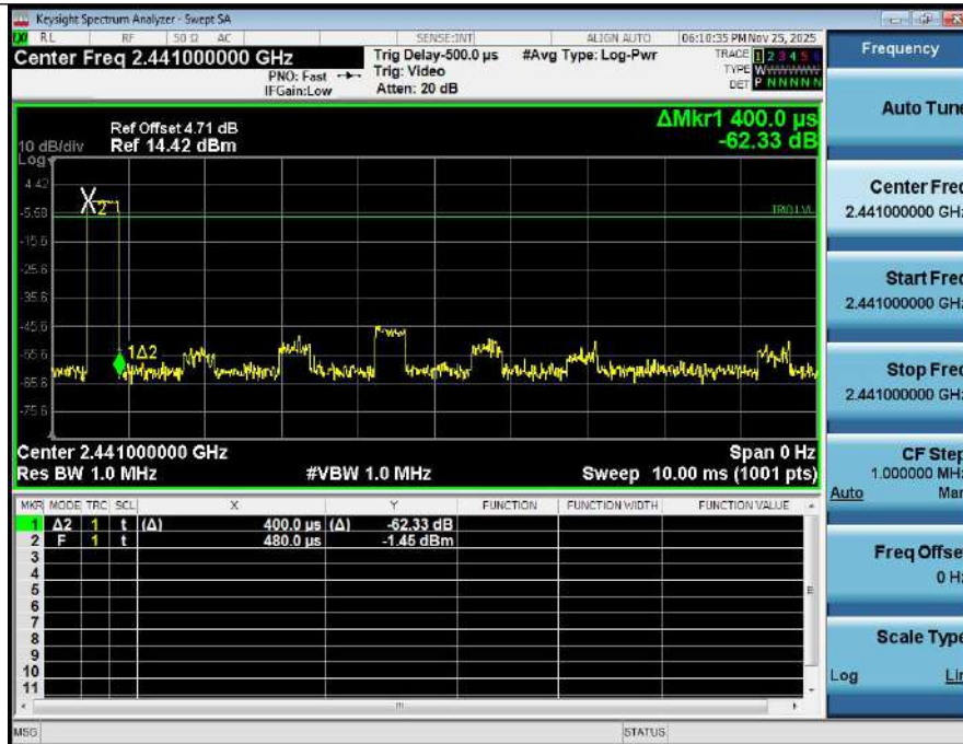
Dwell Time (Hopping) NVNT_ANT1_2-DH1_2441_00_Accumulated
