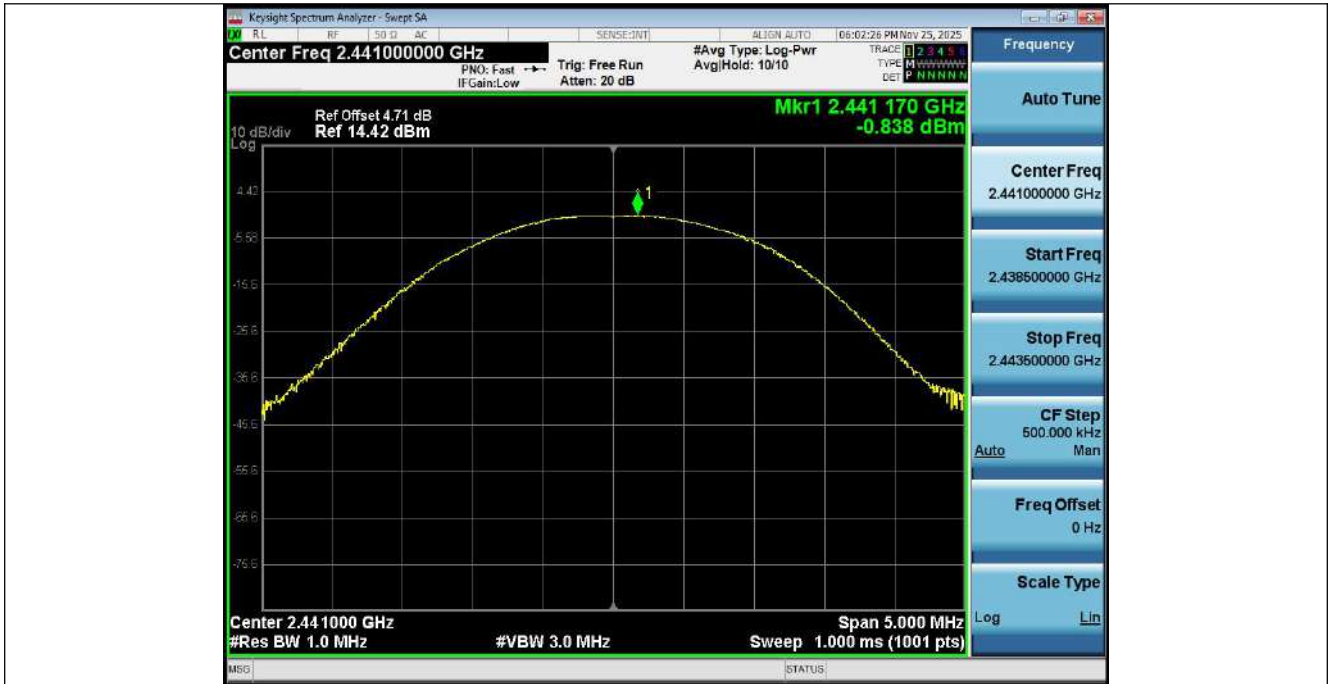
Peak Output Power NVNT_ANT1_2-DH1_2480_00
