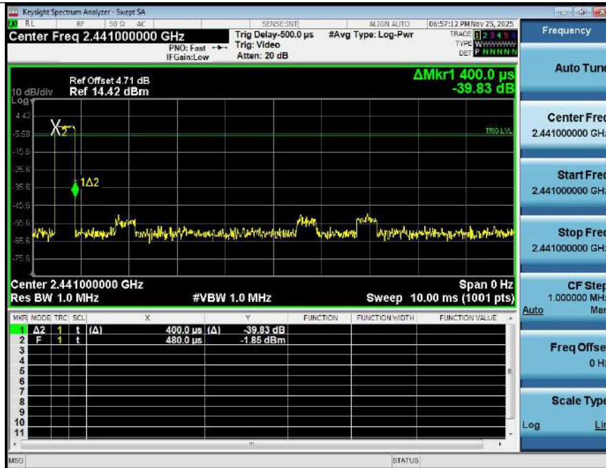
Dwell Time (Hopping) NVNT_ANT1_3-DH1_2441_00_Accumulated
