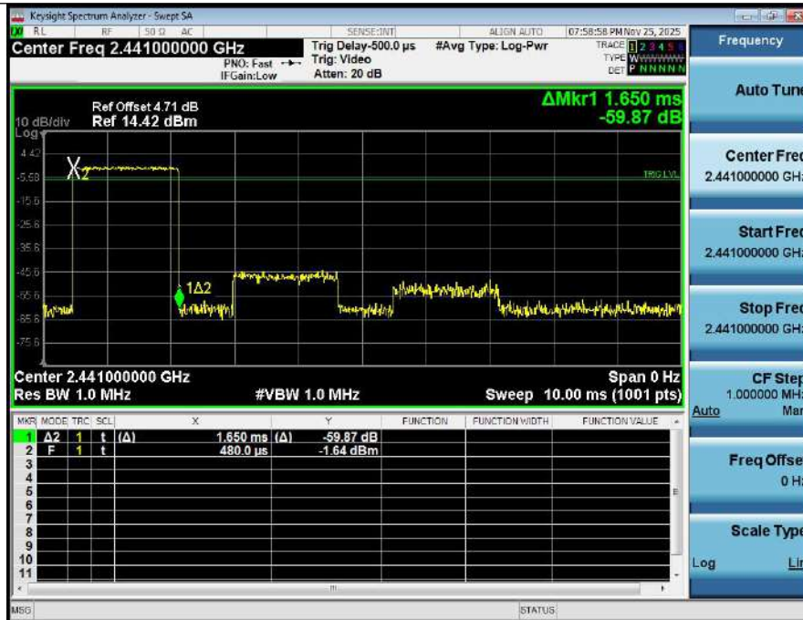
Dwell Time (Hopping) NVNT_ANT1_3-DH3_2441_00_Accumulated
