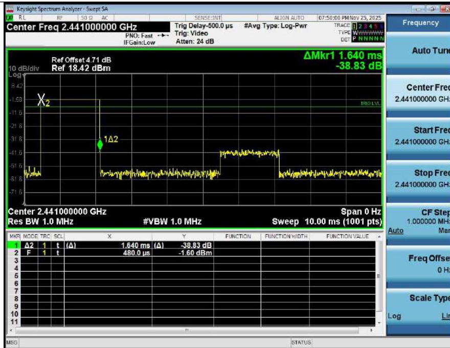
Dwell Time (Hopping) NVNT_ANT1_1-DH3_2441_00_Accumulated
