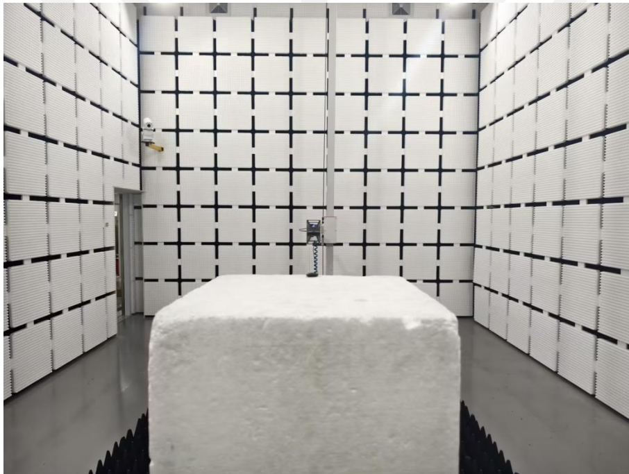
Spurious Radiation Emissions Test (> 1G)
