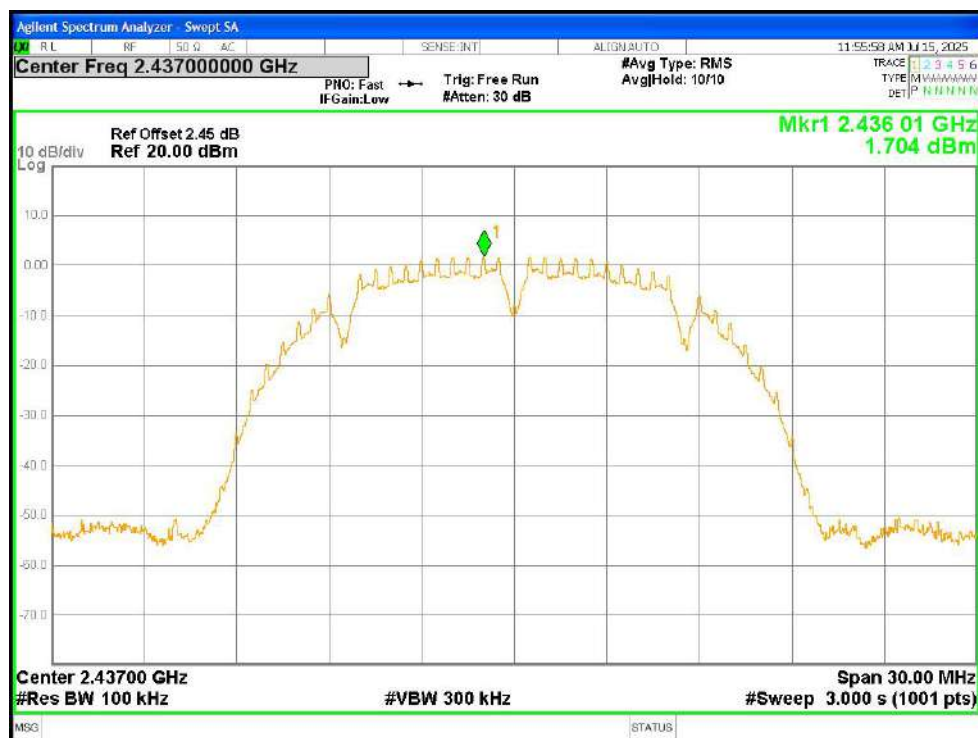
Tx. Spurious NVNT b 2437MHz Ant2 Ref
