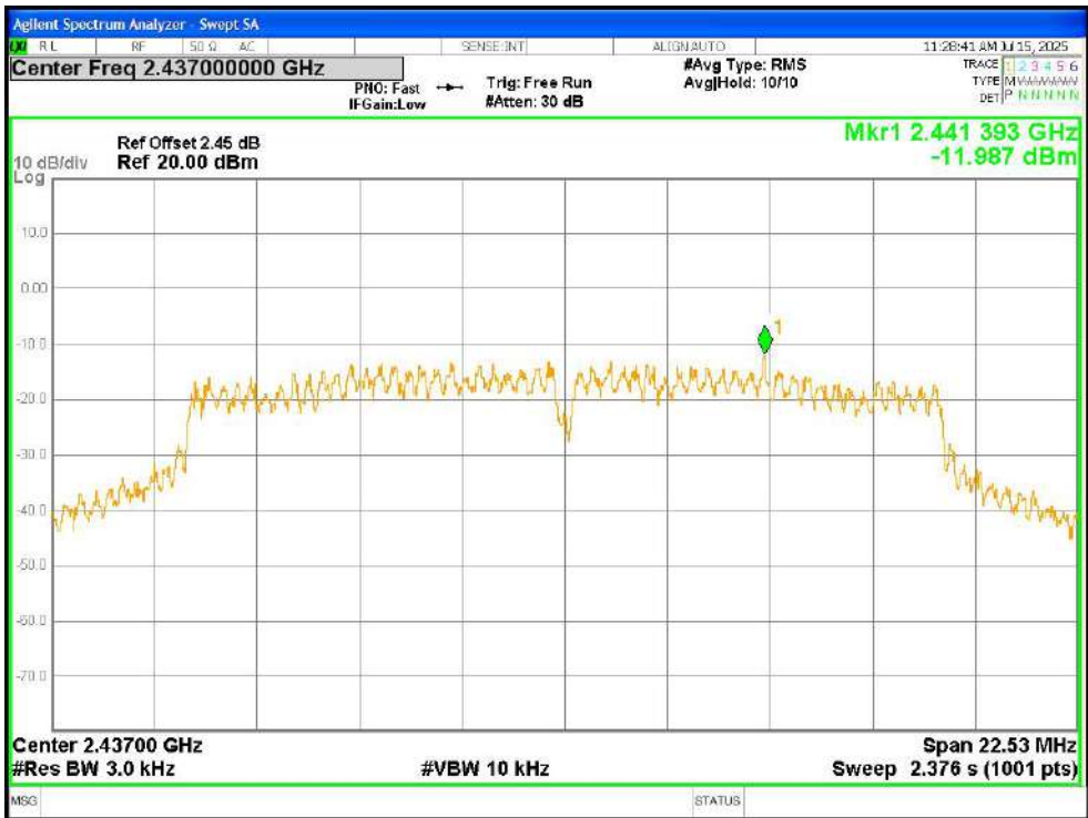
PSD NVNT g 2437MHz Ant2
