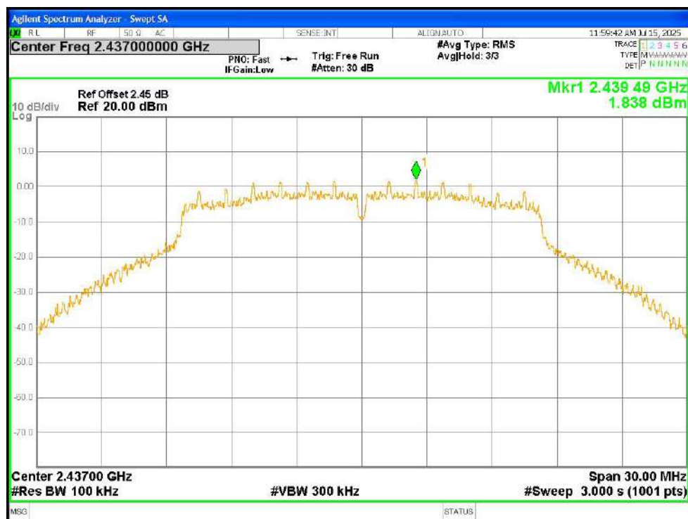
Tx. Spurious NVNT g 2437MHz Ant2 Ref
