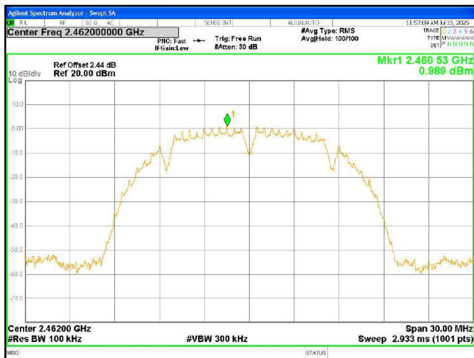
Tx. Spurious NVNT b 2462MHz Ant2 Ref
