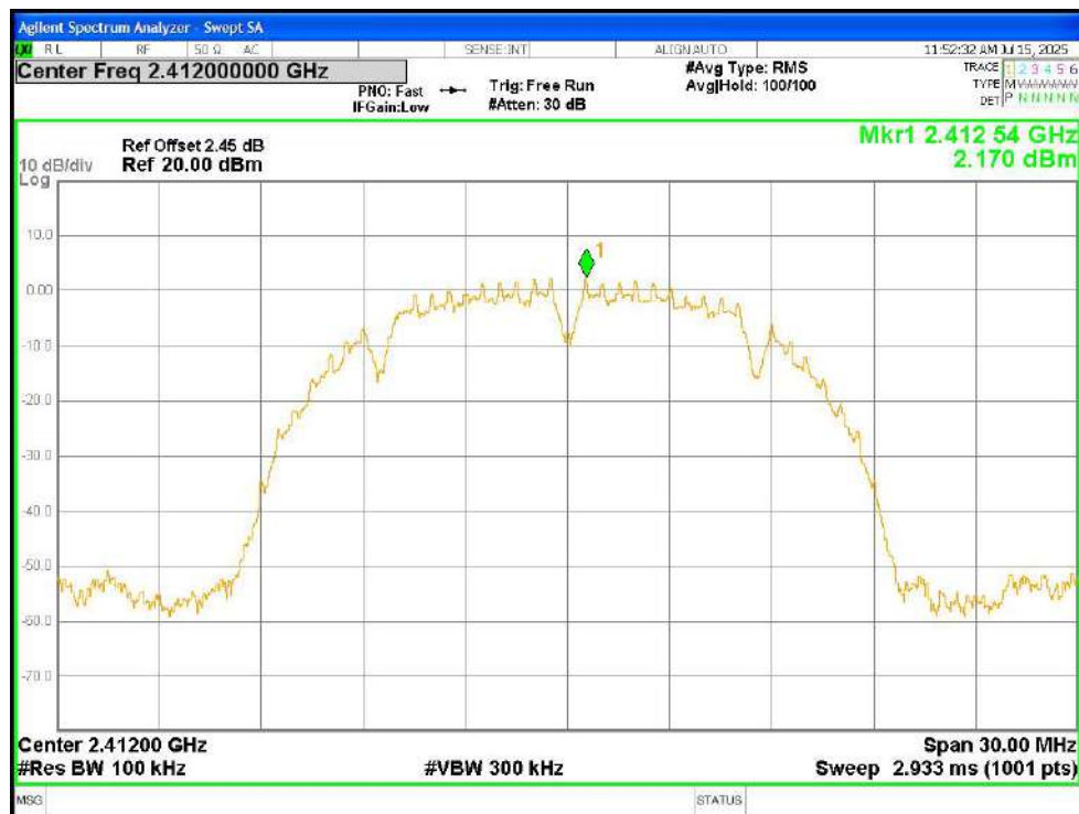
Tx. Spurious NVNT b 2412MHz Ant2 Ref
