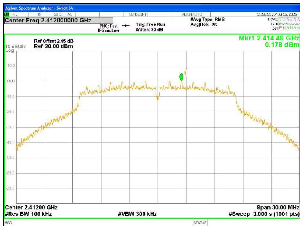
Tx. Spurious NVNT g 2412MHz Ant2 Ref
