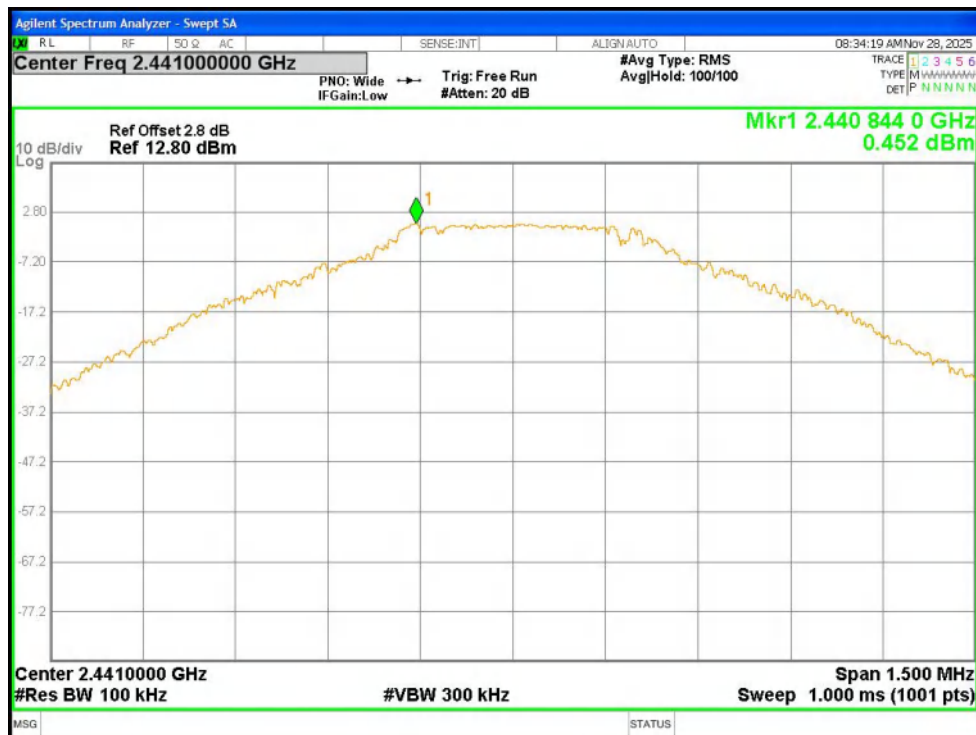
Tx. Spurious NVNT 1-DH5 2441MHz Ant1 Ref
