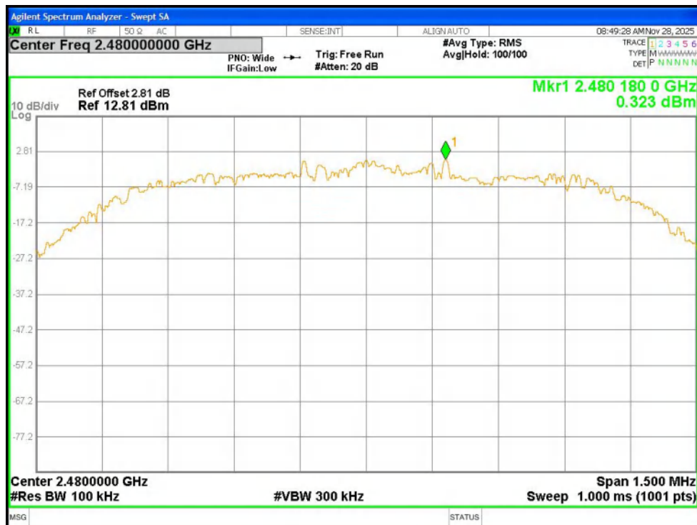
Tx. Spurious NVNT 3-DH5 2480MHz Ant1 Ref
