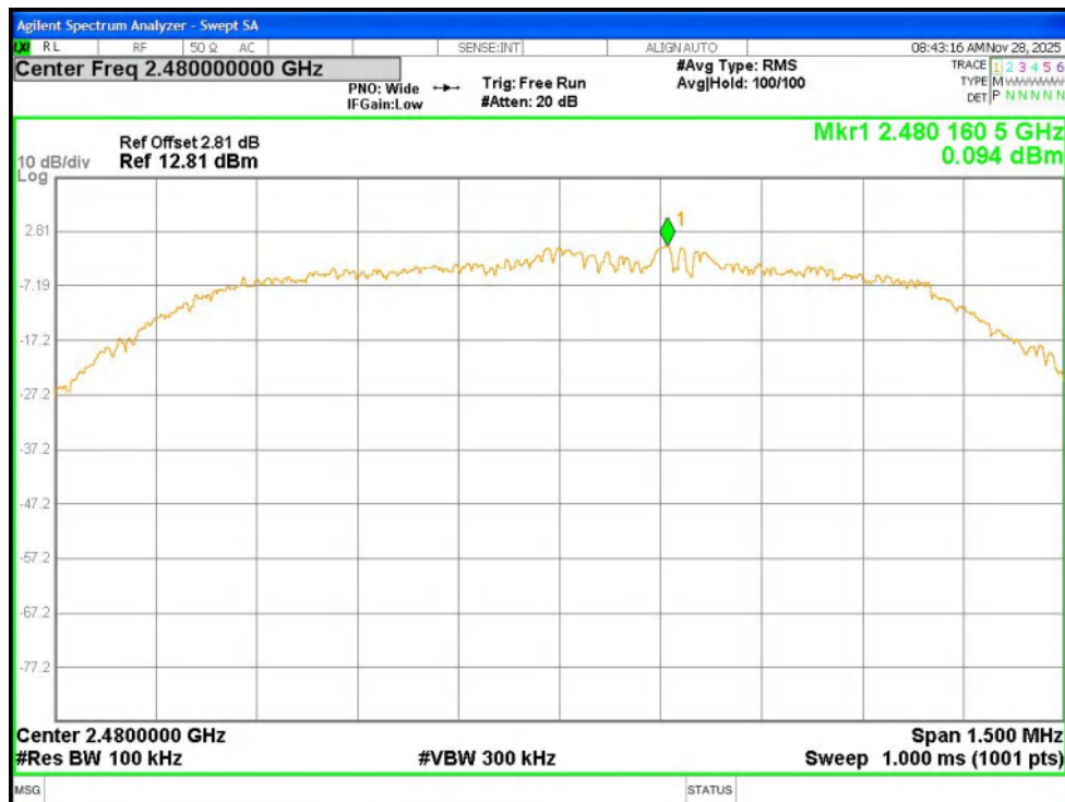
Tx. Spurious NVNT 2-DH5 2480MHz Ant1 Ref
