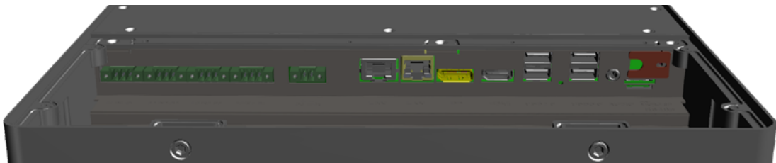
Internal Connectors of the Intercom Solution (11.6" as example)
