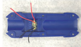
Photo from bottom (After connecting only the lead wire to the base terminal)
