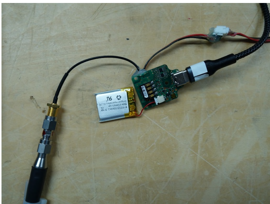
Photograph 2: Set-up for Antenna Port Conducted Emission of Transmitter, EUT
