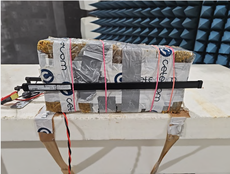
Photograph 5: EUT test setup in the anechoic chamber < 30 MHz, TXRX-mode, close up view_EUT elevation 90°
