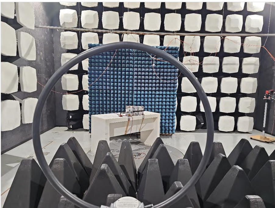
Photograph 6: EUT test setup in the anechoic chamber < 30 MHz, TXRX-mode, overview_EUT elevation 90°
