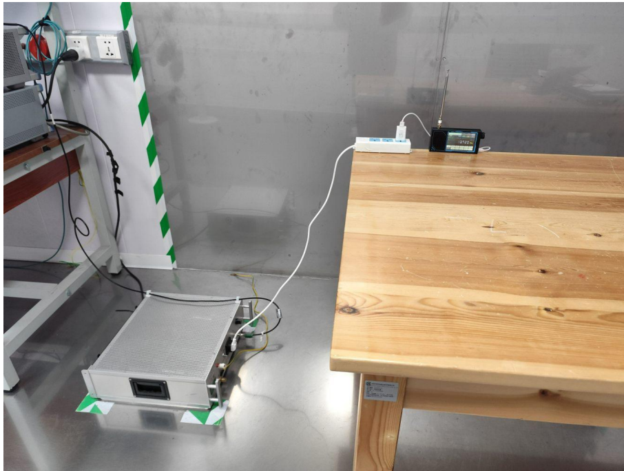
Conducted Emission at AC power line
